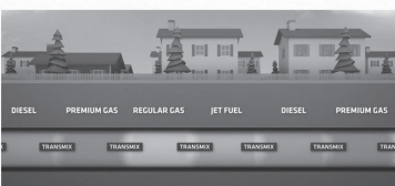
PIPELINE COMPANIES USE BATCHING LINES
